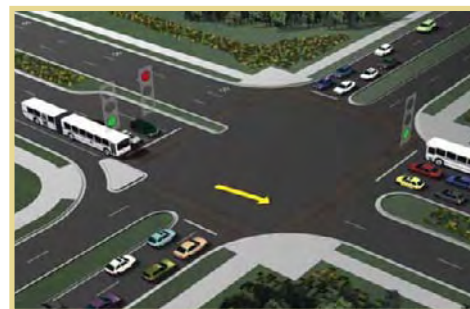
Transit preemption allows buses to continue through an intersection while regular traffic is stopped.
